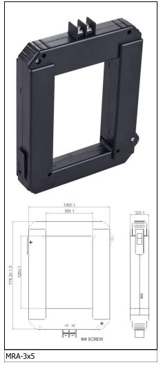
Unlike standard 5A CTs, MRA Current Transformers do not produce high voltages when opened. They generate a low energy mA signal level and no special protection and/or shorting blocks are required. Maximum open secondary voltage is clamped at about 7V ac.
