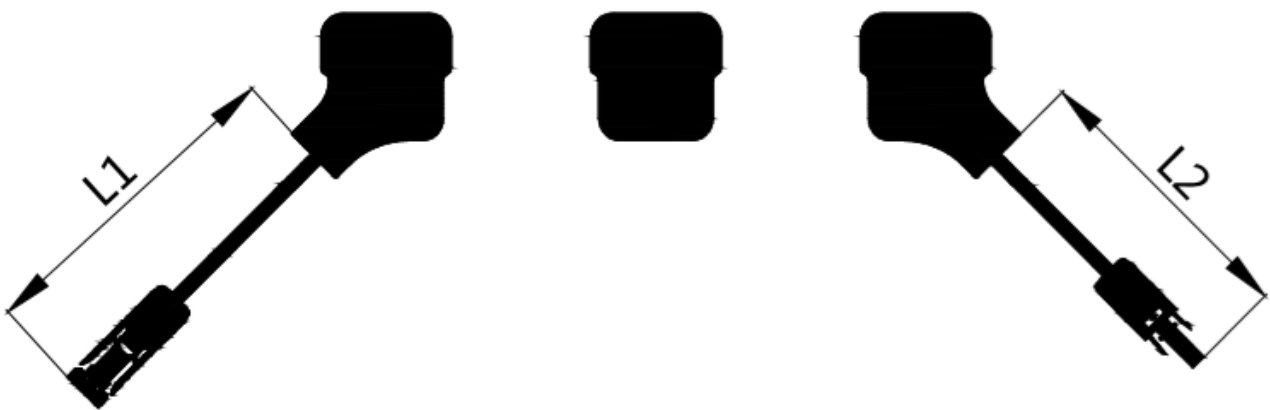
Figure 11 (2): The half-cut module/SWAN bifacial module junction box
