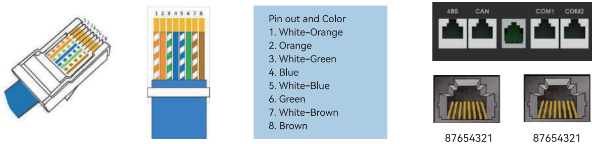
Figure 2-2 CAN, RS485, COM1, COM2 interface definition
